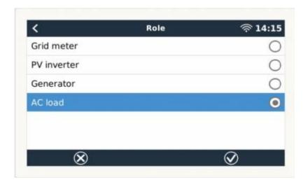
In GX device firmware version 2.80 and later - They can also be used for other purposes e.g. to measure specific, arbitrary AC loads or circuits for example. However it should not be considered a replacement to having a Victron inverter / charger. Attempting to use other brand battery inverters and trying to substitute their lack of data connectivity to the GX device by using energy meters will not work as expected.
